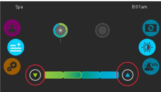
By pressing the up/down arrows on either side of the speed bar will adjust your swim pump speeds in that direction in small increments.
