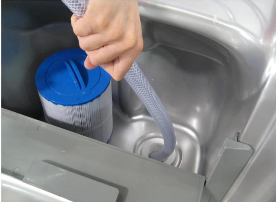
Figure 10. Filling Location in Filter Housing
