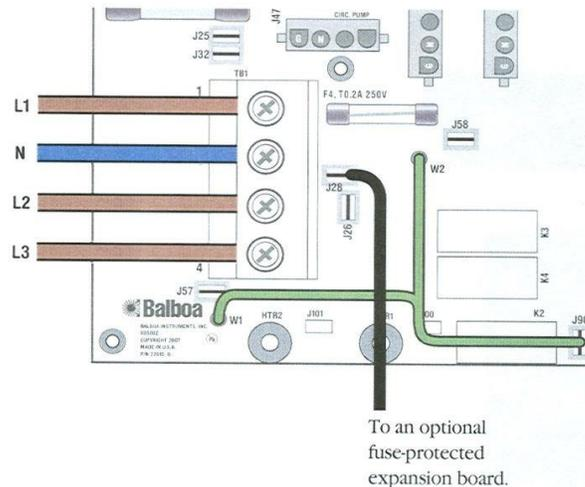
Figure 6. Three Phase Power – TN and TT Electrical Systems
