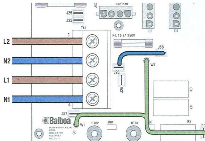
Figure 6. Two Phase Power – TN and TT Electrical Systems
