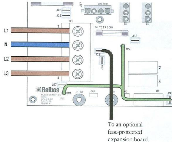
Figure 7. Three Phase Power – TN and TT Electrical Systems
