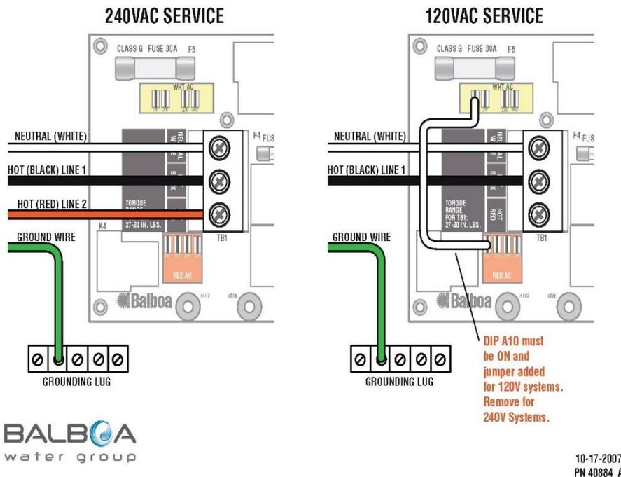
Figure 1. Terminal Connections for 240 V and 120 V Service
