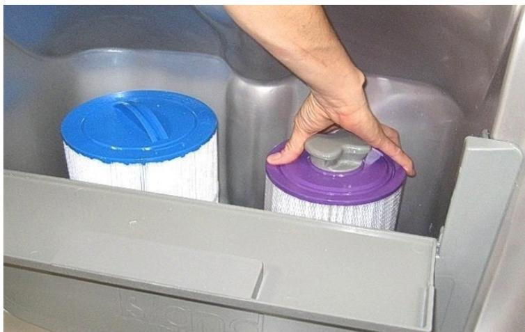
Figure 56. Screw-in Filter Removal
