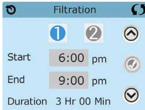
Press “1” to view Filter 1. Press “2” once to view Filter 2. Press “2” again to turn Filter 2 ON or OFF.
