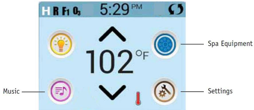
The only item that can be changed on the left side of the Main Screen is the Set Temperature. Touch either the set temperature line or the water temperature to go to the Set Temperature screen. See next page.
