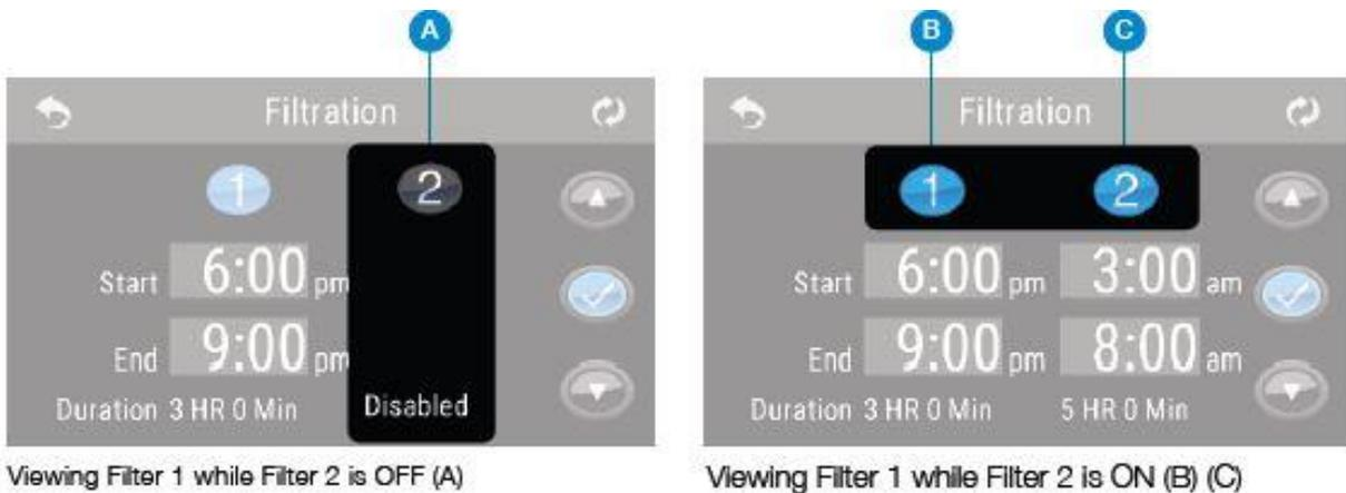
Press “1” (B) to view Filter 1. Press “2” (C) once to view Filter 2. Press “2” again to turn Filter 2 ON or OFF.
