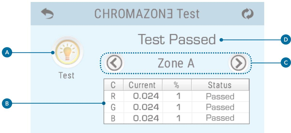
CHROMOZONE™ Test tests the electrical load of all the LEDs in all zones connected to CHROMOZONE™ (E).
