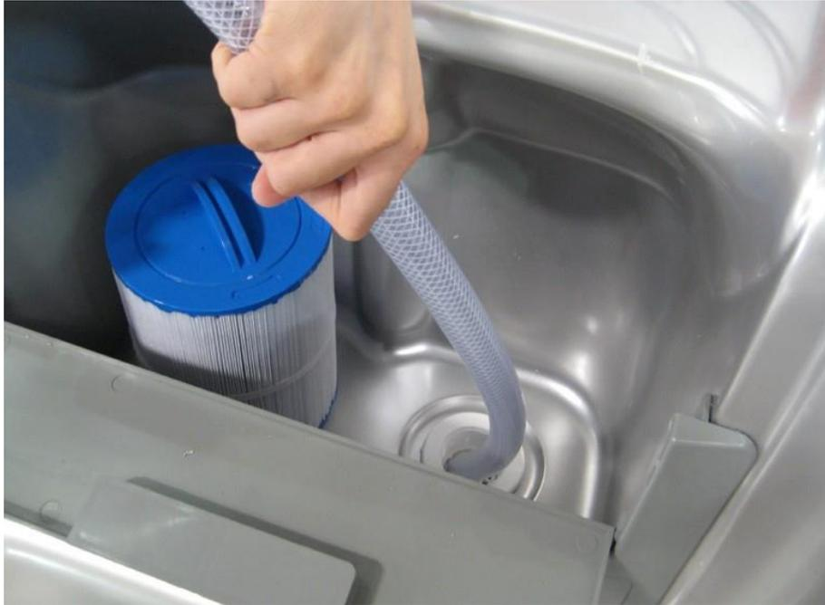
Figure 7. Filling Location in Filter Housing
